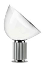
Table lamp providing indirect and reflected light. Reflector in painted aluminium, gloss white on the outside and matt white on the inside. Directionable diffuser in transparent mouth-blown glass. Body in matt black. silver anodized or bronze anodized aluminium. Base in nickel-plated metal. Electric cable of useful length 220 cm, with dimmer switch for ON/OFF and adjustment of the light flow between 10-100%. Plug-in power supply with interchangeable plugs.
